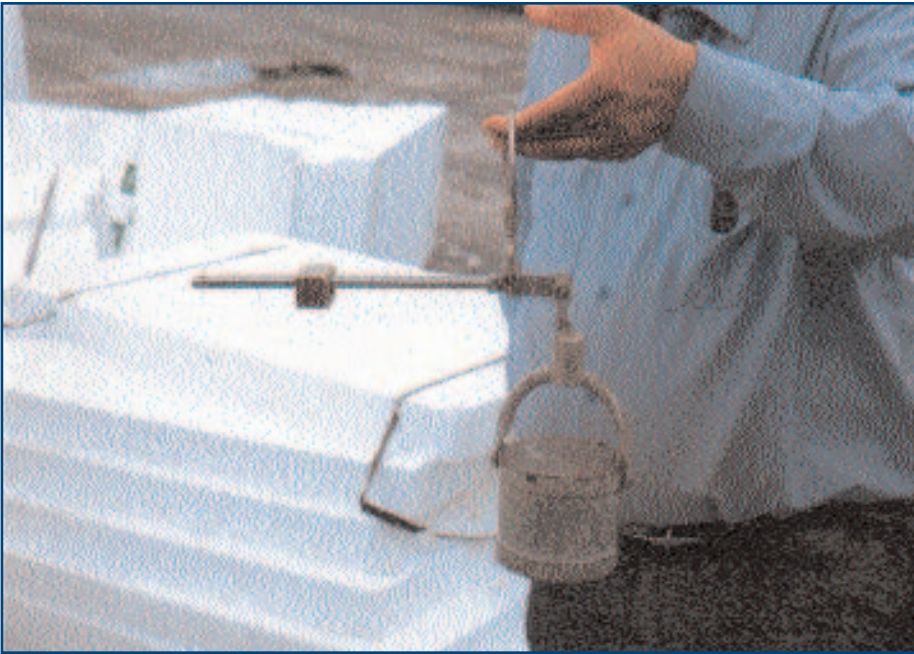
Photo 2: A steel vessel of known volume attached to a balance scale may be used to determine weight.
