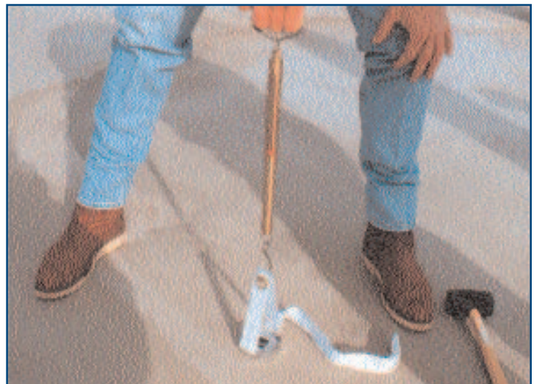
Photos 3 and 4: A spring-type (fish) scale (left) and a custom-fabricated sheet metal holding clamp (right) may be used for pull-out resistance tests on base sheet fasteners.
